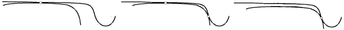
Figure 1.89. Types of contact for a pair of profiles allowing two-point contact: one-point contact, two-point contact and creeping up
