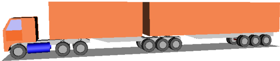
Figure 1.98. 3-unit vehicle: a truck with two semi- trailers
