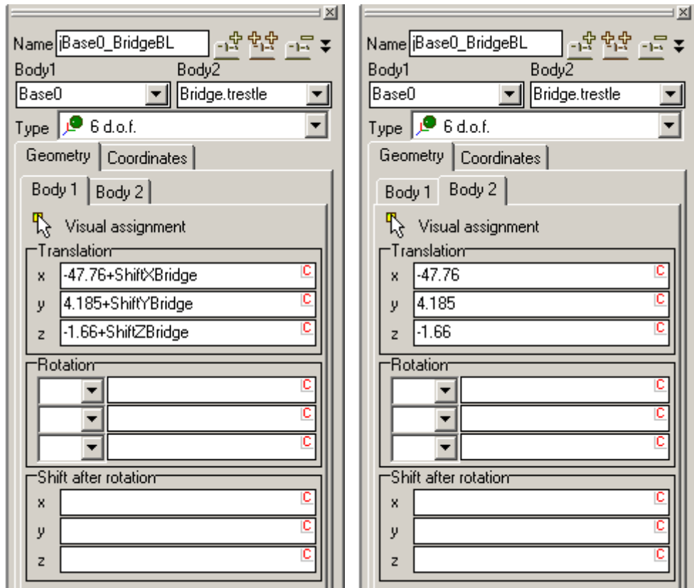
Figure 1.13. Coordinates of the joint point of the left joint on the 1st pier in the SC0 (left) and the local frame of reference of the bridge (right).
