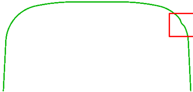
Figure 1.65. Violation of the smoothness of the rail profile in the local section
