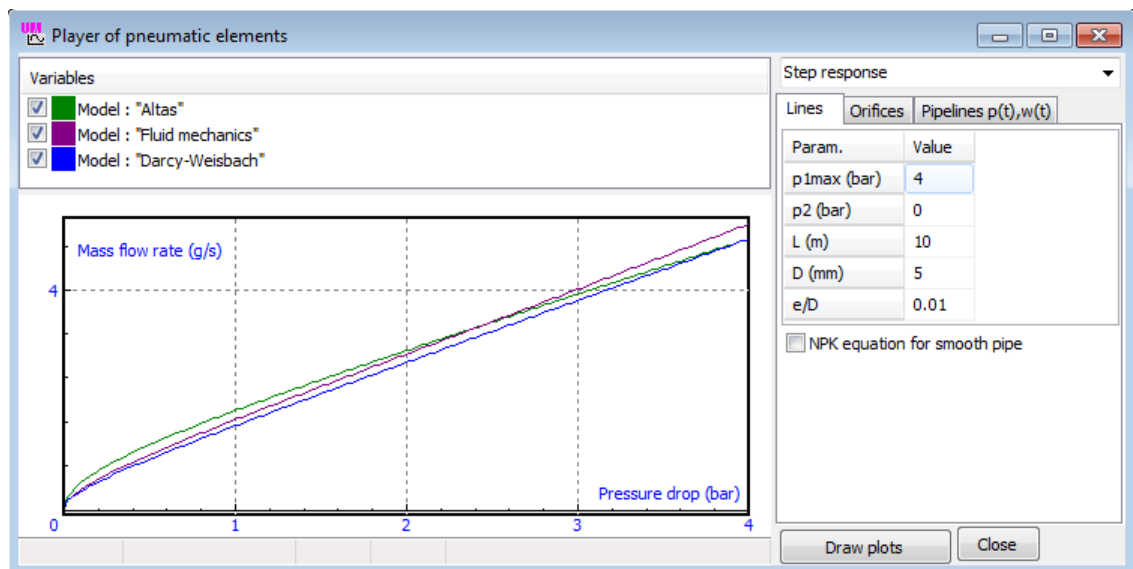
Figure 1.61. Comparison of stationary pipeline models
