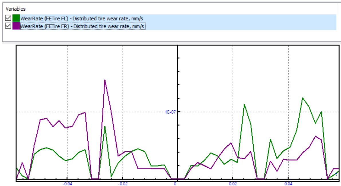
Figure 33.171. Examples of graphs of the distributed wear rate factor when driving on a straight section of the road
