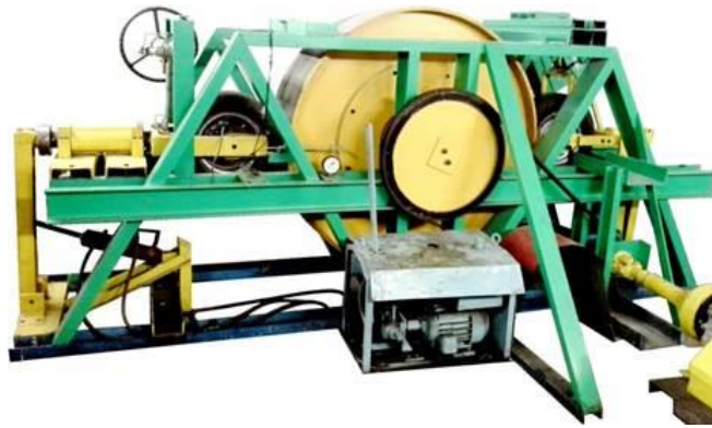
Figure 33.130. Tyre test rig at Irkutsk National Research Technical University
