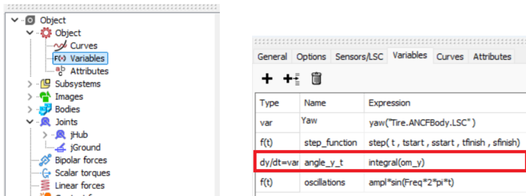
Figure 33.25. List of variables in the wheel template model
