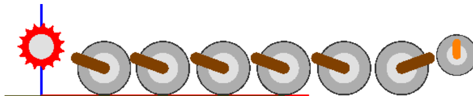
Figure 1.16. Adding idler with tension device
